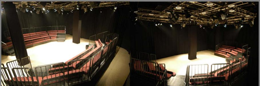
Black surround masking track around a full lighting truss, allowing the venue to be set up in less than 4 hours.
